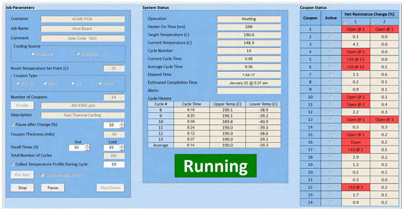
Figure 2: CAT analyzes all areas of the PCB for reliability.
