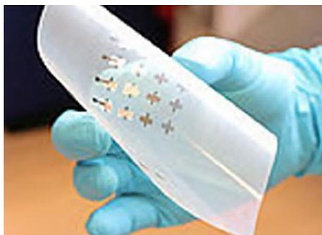
The Trinity College researchers, from the groups of profs. Jonathan Coleman and Georg Duesberg, used standard printing techniques to combine graphene nanosheets as the electrodes with two other nanomaterials, tungsten diselenide and boron nitride, as the channel and separator to form an all-printed, all-nanosheet transistor.
