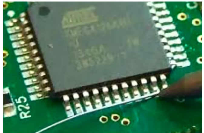
Figure 1: Point-to-point soldering of a QFP.
