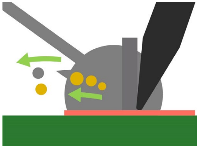
Figure 2: Feeding solder wire too quickly can lead to solder ball formation.
