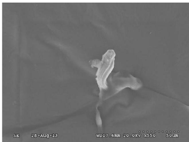
Figure 8: Scanning electron micrographs detailing the appearance of tin whiskers protruding through 2.0 mil thick acrylic coating in the compression region of a bent Alloy 42 base metal coupon.
