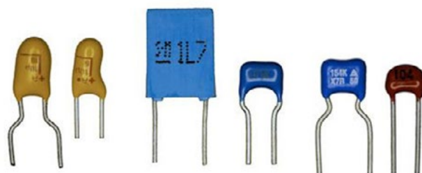
Figure 3: Plated through-hole components.
