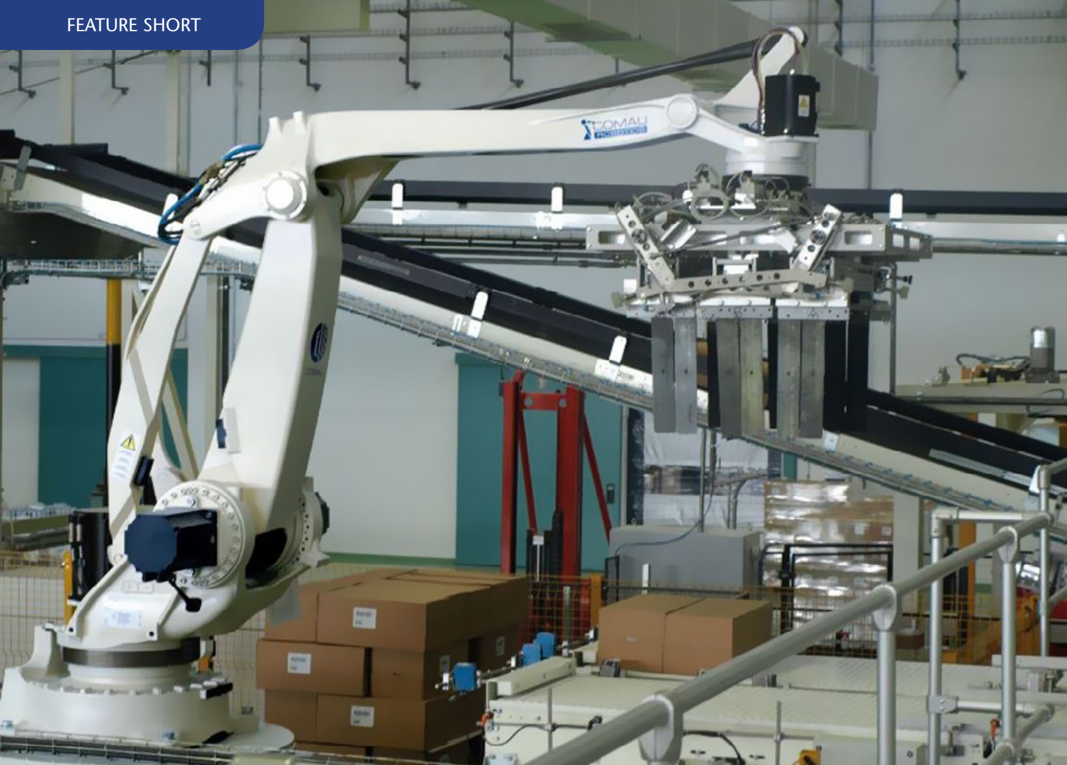
Figure 1: The Comau Smart Pal is used for palletizing and logistics operations.
