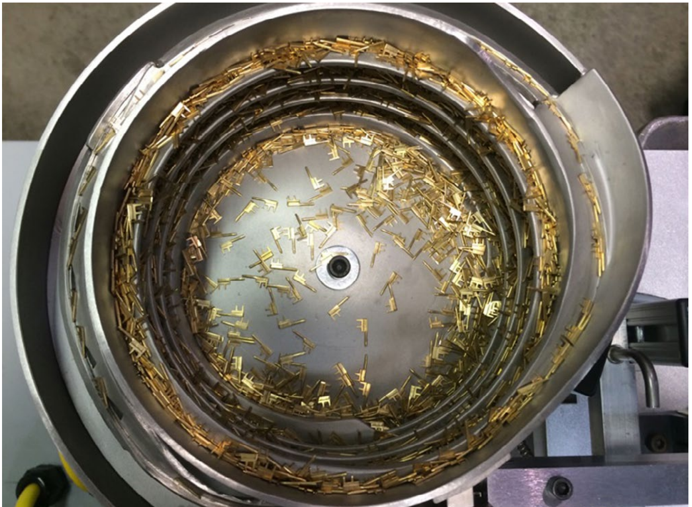
Figure 5: Top view of bowl for automatable pin.
